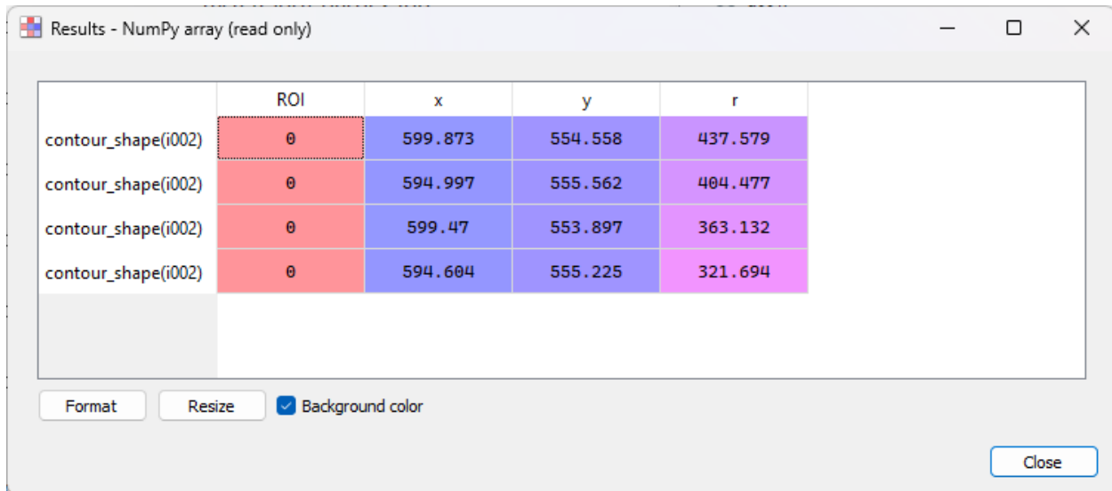
Fig. 60: Select the “Contour detection” tool in the “Computing” menu, with the same parameters as before (shape “Circle”). On this image, there are two fringes, so four circles are fitted. The “Results” dialog opens, and displays the fitted circle parameters. Click “OK”.
